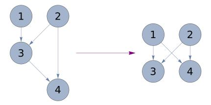
In particular, if you have a situation like the DAG on the left, then we can replace it with the equivalent circuit on the right which has strictly better instruction-level parallelism.
