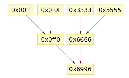
Here's an example of a Boolean chain which computes the XOR of four inputs. We've annotated each node by its truth table, written in hexadecimal rather than binary for brevity. Now we're going to do something quite drastic, which is to forget the whole DAG structure and just represent this by the set of its non-input truth tables.
